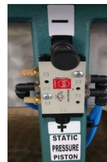
Figure 15 - Pneumatic Pressure Adjuster
