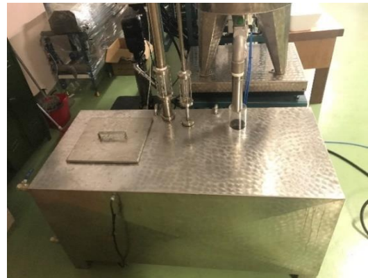
Figure 9 – Main Water Tank
